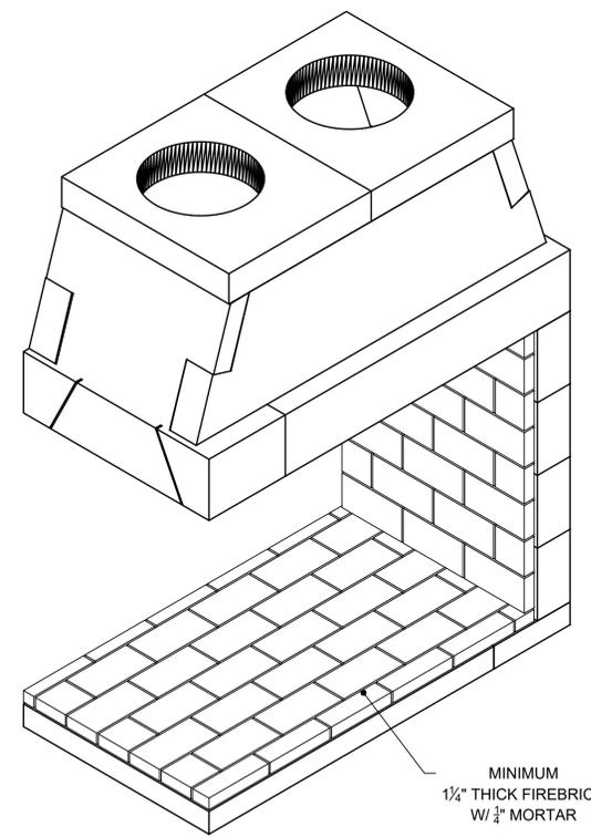
NOTE: IN ORDER TO SUPPORT THE SMOKE DOME OF THIS FIREBOX, A STRUCTURAL STEEL SUPPORT FRAME MUST BE DESIGNED AND APPROVED BY A STRUCTURAL ENGINEER. SMOKE DOME WEIGHT EXCLUDING MORTAR AND EXHAUST COMPONENTS IS 672 LBS.
